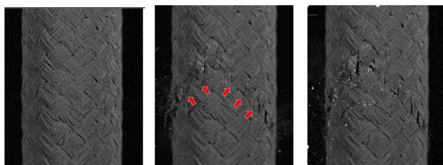
Fig. 11. 45° 3-ply biaxial hoop burst test captured using a high-speed camera at different times throughout the test (pristine sample, initial fracture, and highest strength). The red arrows indicate the location of microcracks initiated early during the fracture.
